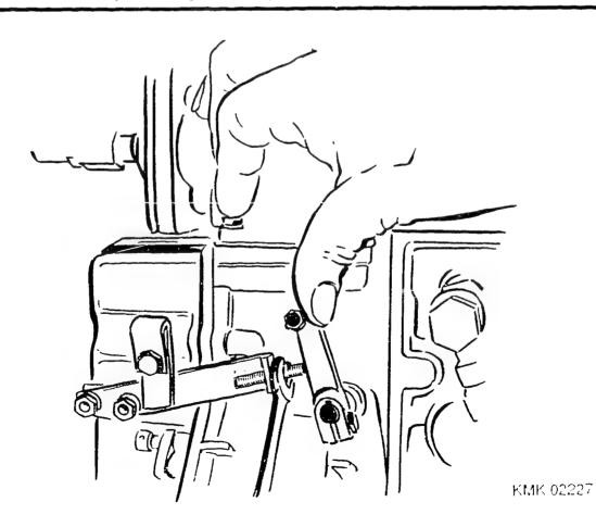
GOVERNORS WITH MANIFOLD—PRESSURE COMPENSATOR (LDA) AND BUILT—IN FULL—LOAD STOP
